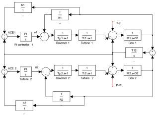
Fig.1 block diagram of a two area power system with the controller
