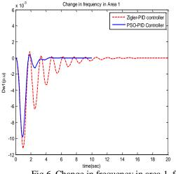
Fig 6. Change in frequency in area 1 for a step load of 1% at area 2
