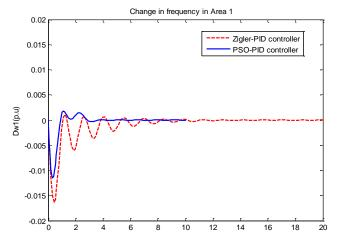
Fig.3.Change in frequency in area 1 for a step load of 1% at area 1
