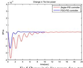
Fig 5.Change in tie line power for a step load of 1% at area1
