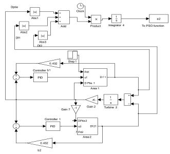
Fig.2 block diagram of a two area power system with the optimal controller and PSO function
