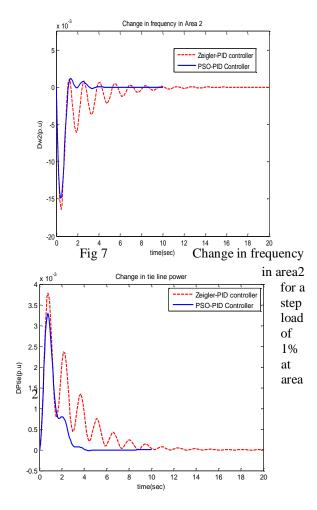
Fig 8.Change in tie line power for a step load of 1% at area2
